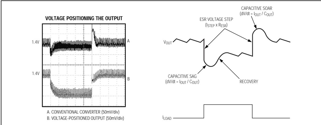
Figure 11. Voltage-Positioning Transient Response
