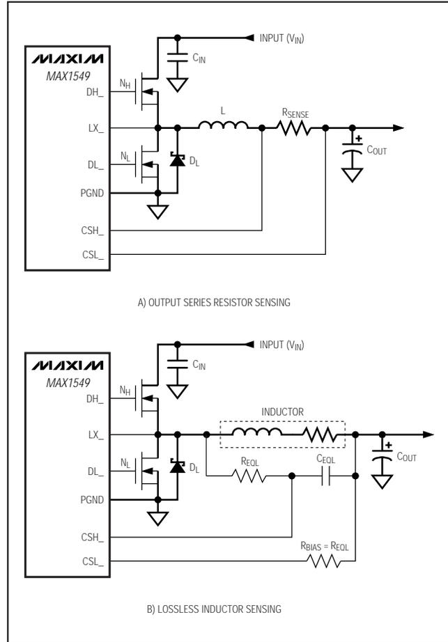
Figure 8. Current-Sense Configurations
