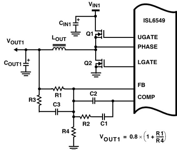
FIGURE 7. OUTPUT VOLTAGE SELECTION OF THE SWITCHER ( $V_{OUT1}$ )
