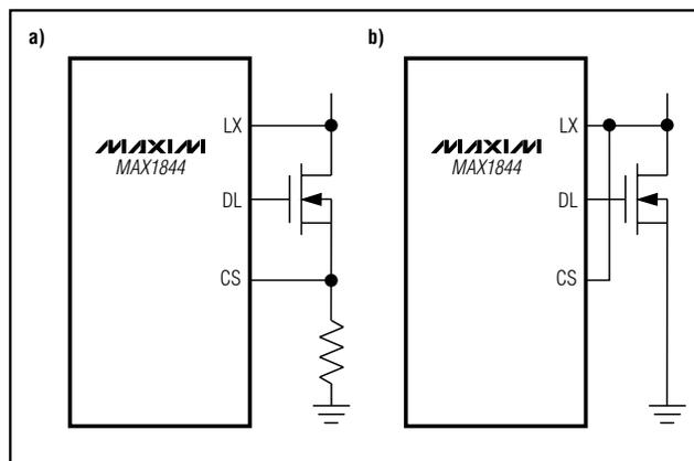
Figure 8. Current-Sense Circuits
