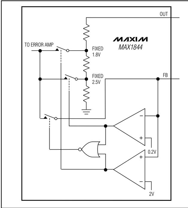
Figure 6. Feedback Mux
