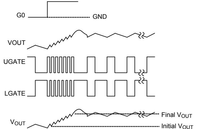
Figure 6. Output Voltage Up Transition with Overshooting
