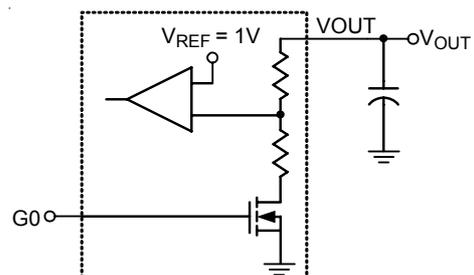
Figure 3. Output Voltage Selection by G0 Input
