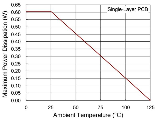
Figure 9. Derating Curves for the RT8240A/B/C Package
