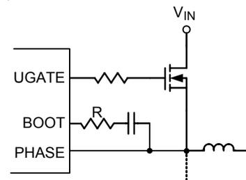
Figure 8. Increasing the UGATE Rise Time
