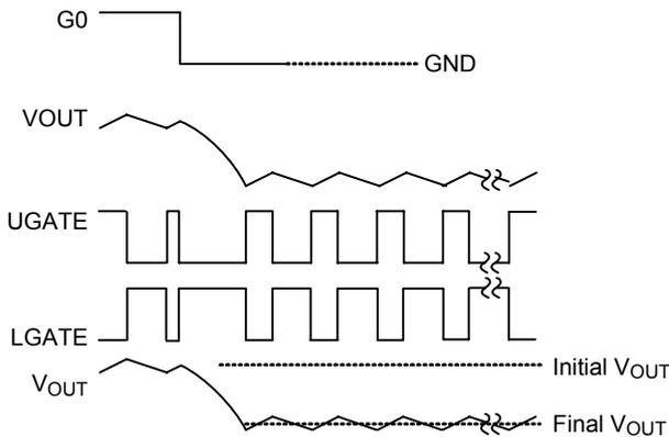
Figure 4. Output Voltage Down Transition
