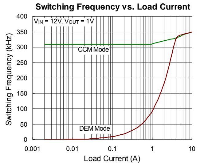
Switching Frequency vs. Load Current
