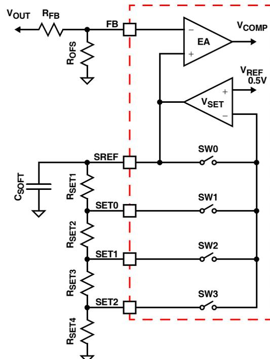
FIGURE 11. ISL95870B VOLTAGE PROGRAMMING CIRCUIT
