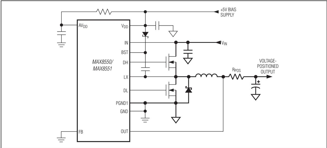
Figure 9. Voltage-Positioned Output
